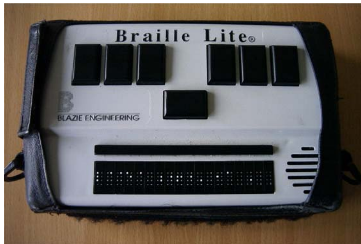
Figure 1: Blaze Engineering's BrailleLite, a Braille-based note-taking device (photo: Hans Schou)
